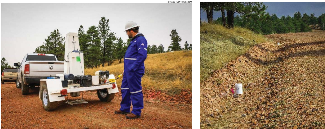
Figure 1. Right: Photo of the EERC seismic acquisition team operating the GISCO ESS850 850-lb seismic weight-drop source along an existing roadway in southwestern Montana. Left: Photo of the EERC's autonomous seismic sensors deployed along the same roadway.
